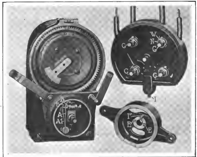
Fig. 5—Details of distributor and breaker construction
